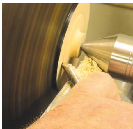
▲ Pic.32 Take light cuts with a small tool. The more you remove the less you will have to hand finish but don't go too far - you don't want to ruin the bowl at this stage
